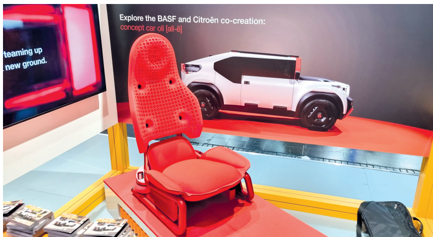
Fig. 5. The joint vehicle study "Oli" from Citroën and BASF is intended to show how future electric vehicles can become more sustainable and affordable. For improved recyclability, the seat is made completely of a mono-material. © Hanser/F. Streifinger
