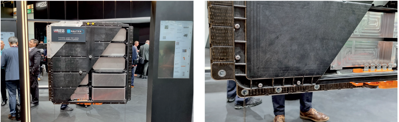
Fig. 3. The battery demonstrator is based on the battery of the ID.3. The housing was manufactured entirely of plastic in a single-stage process. For protection, it was reinforced with a continuous fiber composite at specific points. © Hanser/F. Streifinger
