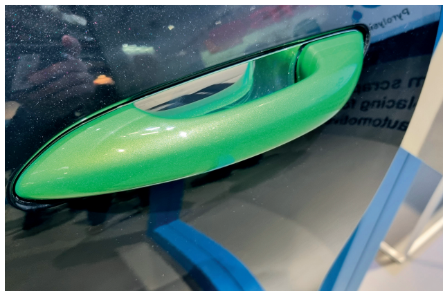
Fig. 7. Tires to door handles – the PA6 used to produce the Mercedes Benz S-Class component is made from pyrolysis oil from old tires and biomethane.
