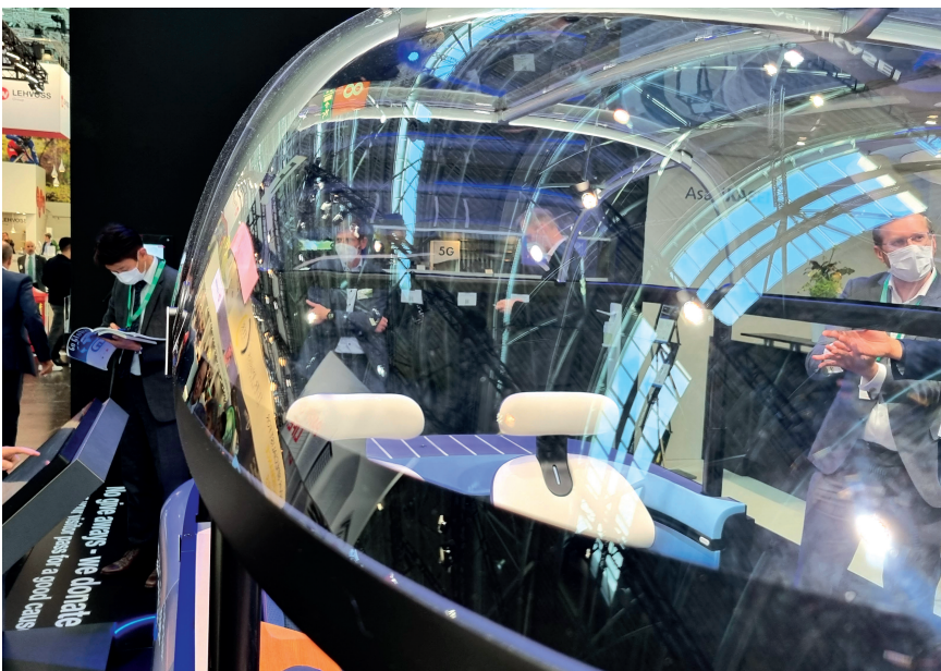
Fig. 4. The dome of Asahi Kasei's concept car is made of PC. A specially developed coating increases scratch resistance and weatherability, thereby meeting the requirements for wind-screens. © Hanser/F. Streifinger
