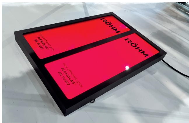
Fig. 6. Tail lamps with low resource and energy consumption are made possibly by a PMMA from Röhm. The material is more transmissive for red light, permitting the lamps to be built using fewer and lower-luminosity LEDs. © Hanser/F. Streifinger
