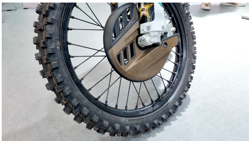
Fig. 2. Exciting features of the brake disk protection are both the production process as well as the material used: the applied jointing method creates a molecular bond between thermosets and thermoplastics. The thermoplastic used is a bio-based PA from Akro-Plastic. © Hanser/F. Streifinger
